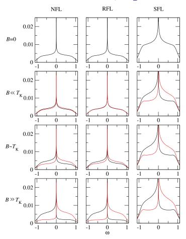
**Figure 4.** T = 0 spectra of the three models for a range of magnetic fields. The magnetic fields are  $B = 10^{-6} \ll T_{\rm K}$ ,  $10^{-5} \sim T_{\rm K}$  and  $10^{-4} \gg T_{\rm K}$ . Red curves: spin up,  $\sigma = \uparrow$ , black curves: spin down,  $\sigma = \downarrow$ .
